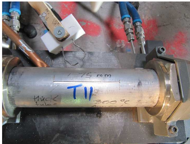
Figure 11-4 Machined slot on top of the tube for controlled failure
