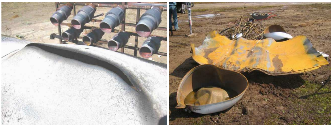
Figure 2-1 Vessel failures from experiments (left: partial failure in fish mouth pattern ; right: total failure) (Birk et al., 2006a)
