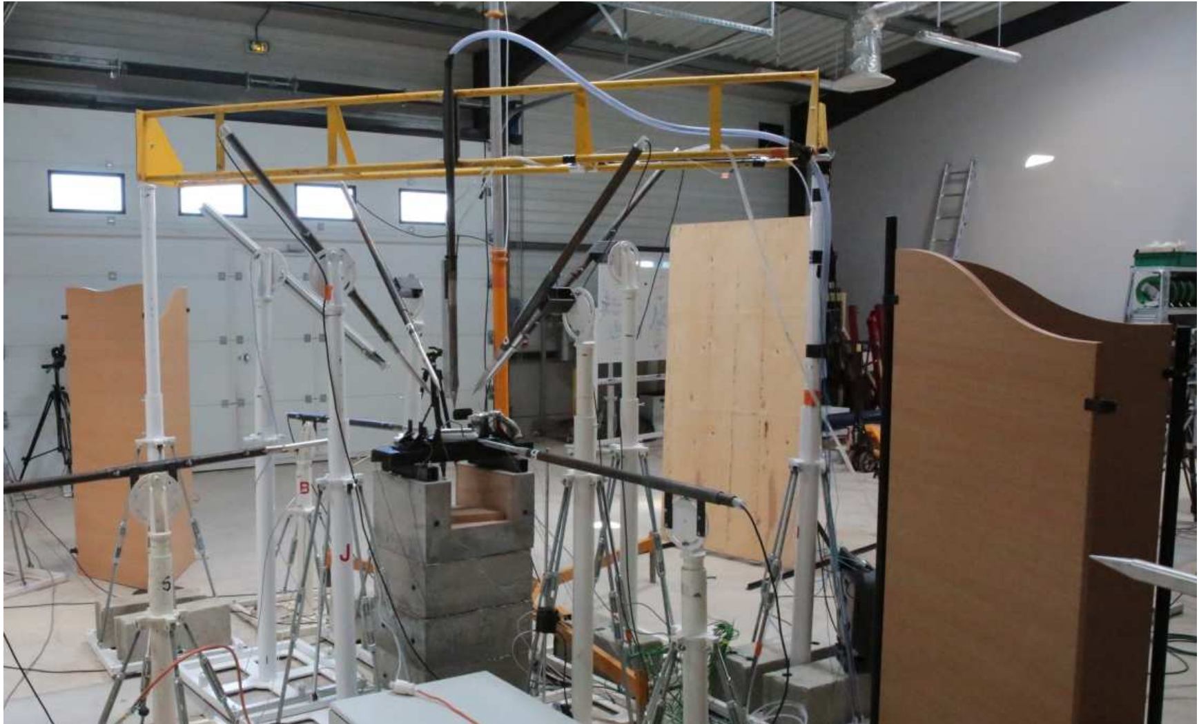
Figure 4-9 Photo of the blast gages setup
