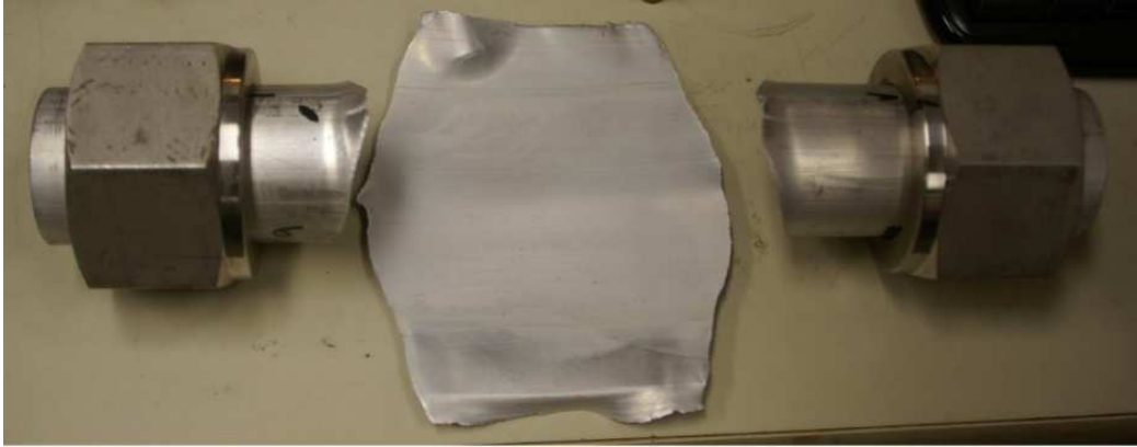
Figure 5-5 Full opening: catastrophic failure with flattening of the tube and separation into 3 pieces (P_{fail} = 20\text{bar}, \Phi_{liq} = 60\%, \text{wall thickness} = 0.9\text{mm})
