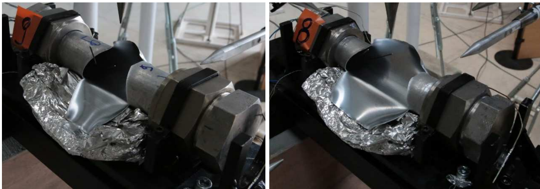
Figure 5-9 One-sided openings (left: P_{fail} = 19.0\text{bar} , \Phi_{liq} = 56\% , L_w = 50\text{mm} ; right: P_{fail} = 12.5\text{bar} , \Phi_{liq} = 59\% , L_w = 100\text{mm} )
