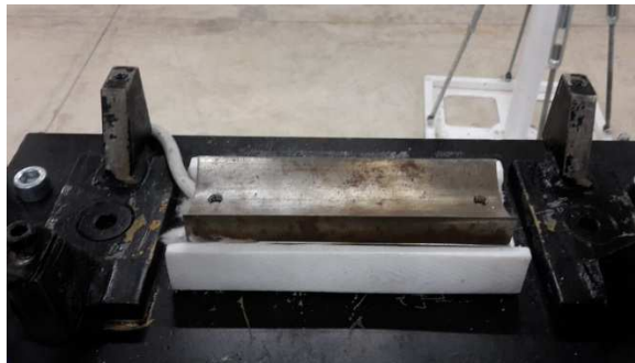
Figure 4-5 Electric heater plate, machined to match the shape of the tube
