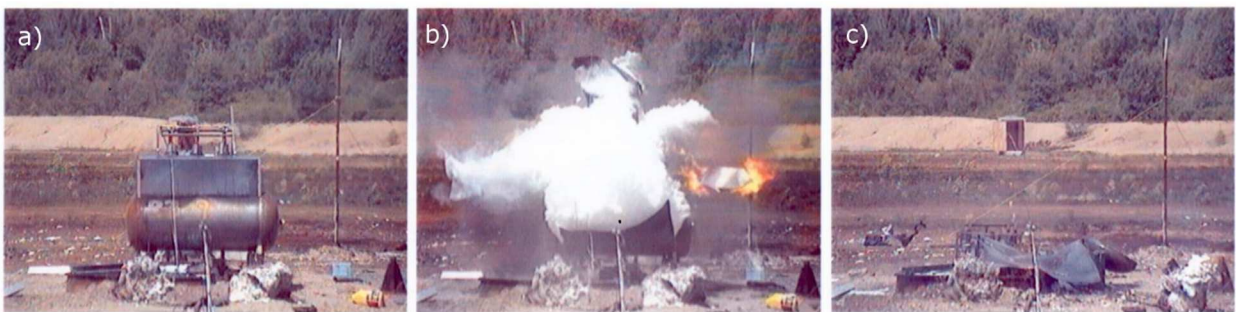
Figure 2-9 Catastrophic failure of a 1m³ experimental propane vessel (a) vessel before explosion ; b) explosion and radial propagation of the crack through the ends; c) after explosion, vessel flat on the ground) (Birk et al., 2007)
