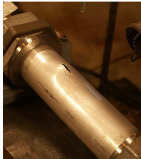
Figure 5-4 Partial failure with fish-mouth type of opening ( P_{fail} = 15\text{bar} , \Phi_{liq} = 60\% , wall thickness = 0.9mm)
