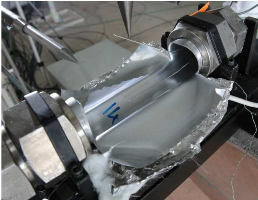
Figure 5-7 Full opening: catastrophic failure with flattening of the tube ( P_{fail} = 18.3\text{bar} , \phi_{liq} = 18\% , L_w = 150\text{mm} )
