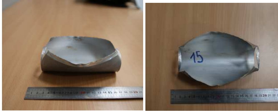
Figure 5-8 Full vessel opening from air burst ( P_{fail} = 15.5\text{bar} , Air, L_w = 150\text{mm} )
