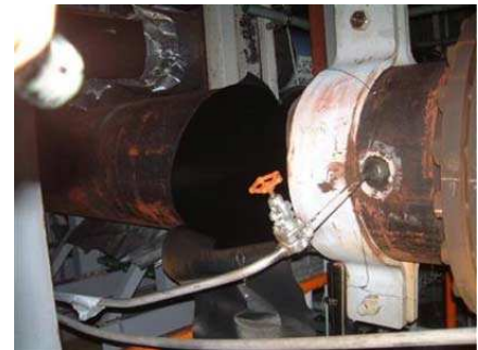
Figure 2-5 Ruptured pipe of the reactor, Japan 2004
