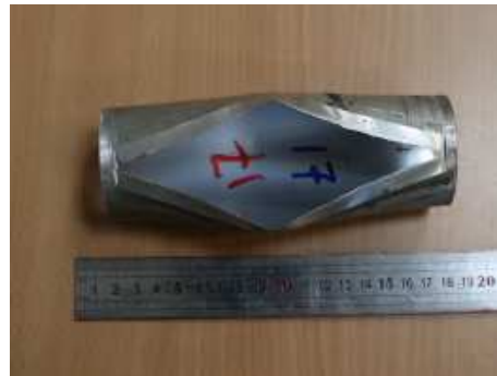
Figure 5-11 Liquid overfilled test (left P - T diagram ; right: tube not fully open after burst)
