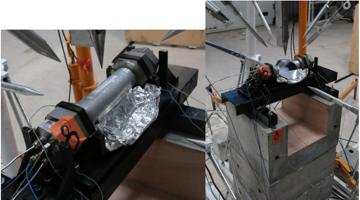
Figure 4-2 Photo of the experimental tube (left: close-up view before experiment; right: view on concrete stand, after burst)
