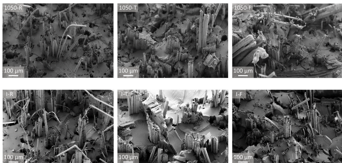
Fig. 8. SEM images of fracture surface of specimens after tensile tests.
