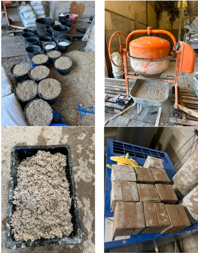
Fig. 2. Manufacturing of biobased concretes (weighing, mixing in the concrete mixer, after mixing and moulding steps).
