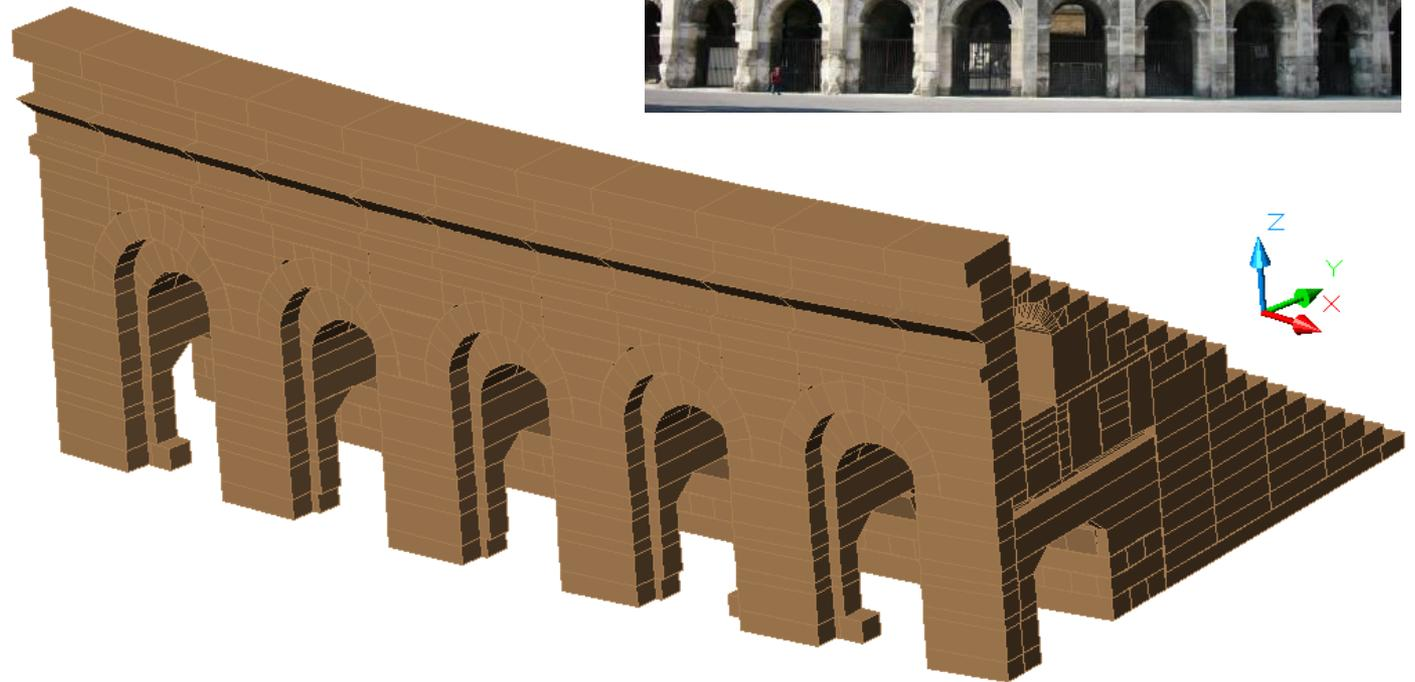
Arena of Nimes, (a) picture taken from outside of the arena, and (b) 3D model generated with AutoCAD software including 2670 blocks for five arches on the first floor.
