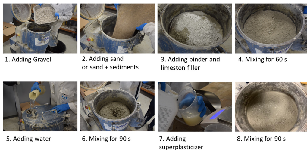
Figure 2. Self-compacting concrete preparation process.
