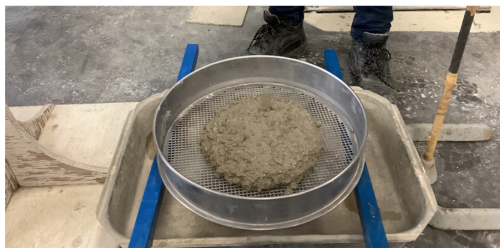
Figure 3. SCC under sieve analysis test.
