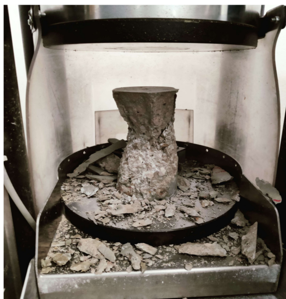
Figure 5. SCC at 28 days under Compressive strength test.
