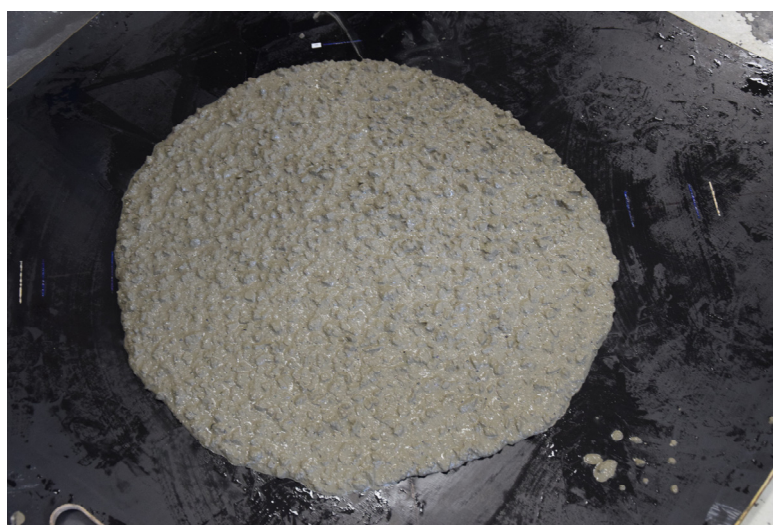
Figure 4. SCC under slump-flow test.
