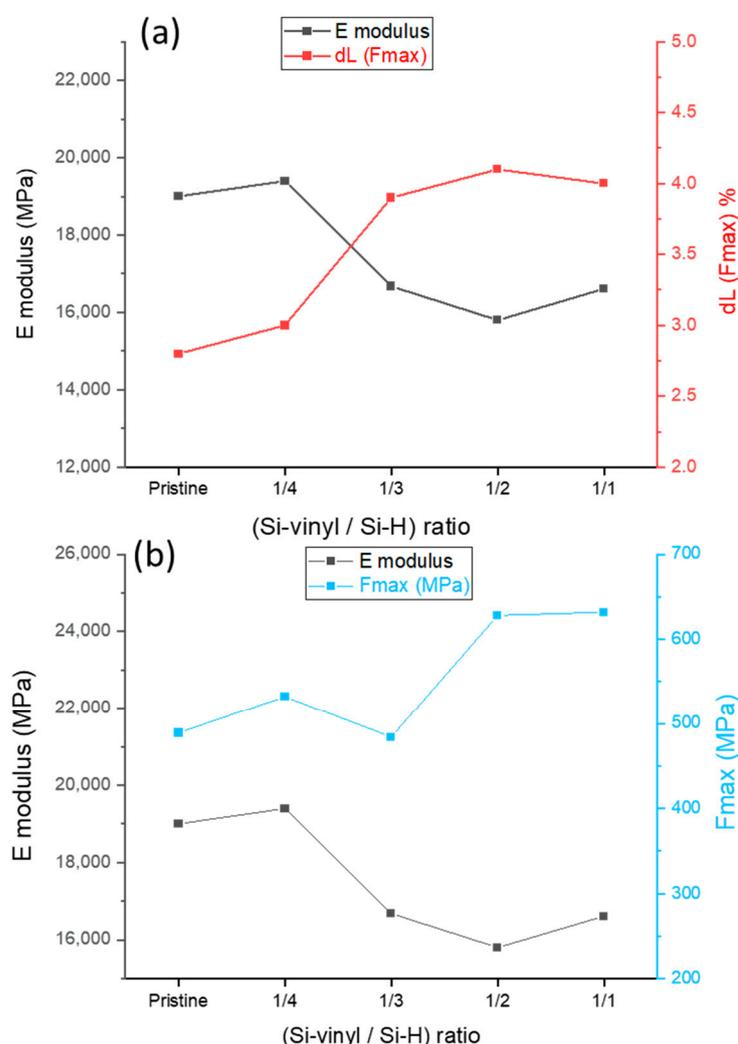
**Figure 5.** (a) Elongation and E modulus, (b) F(max) and E modulus for pristine and coated threads with different Si-H/Si-vinyl ratios.
