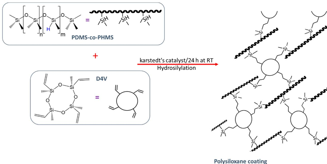
**Figure 6.** Schematic representation of the formation of the cross-linked polysiloxane coating.
