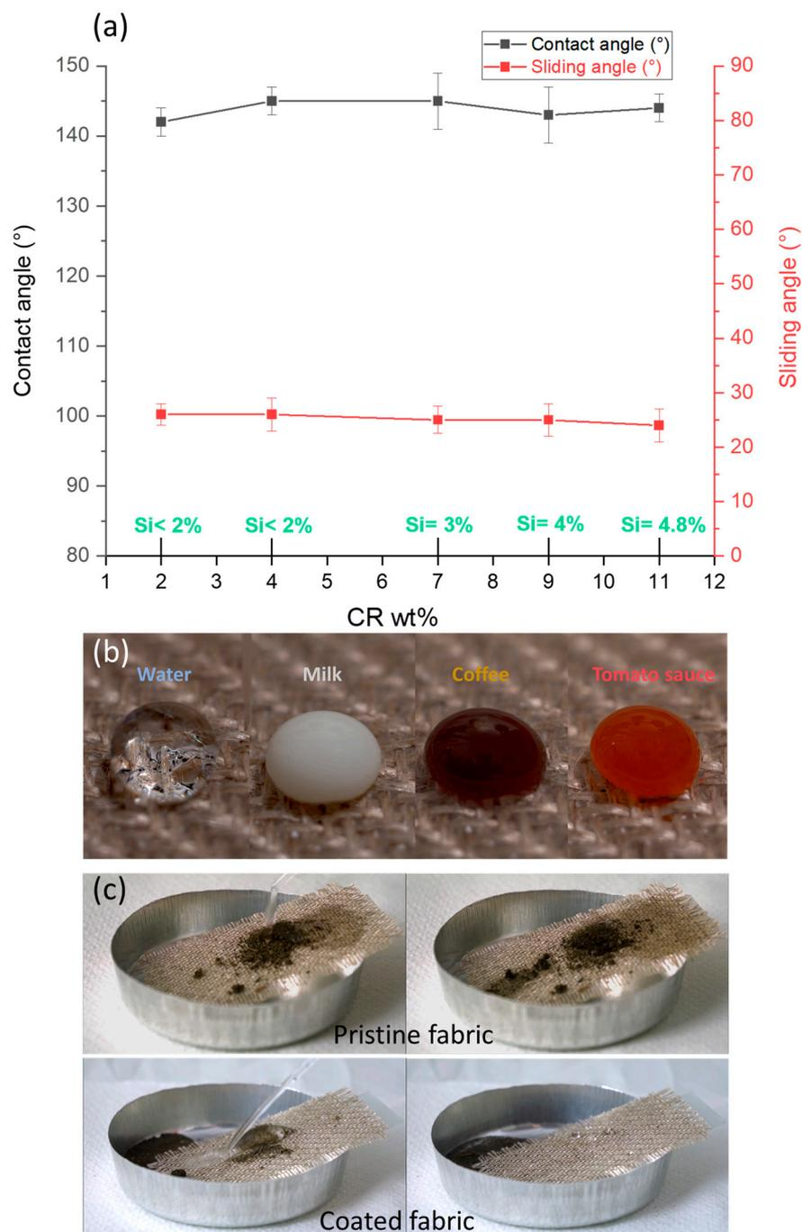
**Figure 4.** (a) Contact and sliding angles for coated samples with different silicone contents. (b) Images of drops of milk, coffee and tomato sauce deposited onto the surface of the coated fabric. (c) Self-cleaning performance of coated fabric for mud stains.
