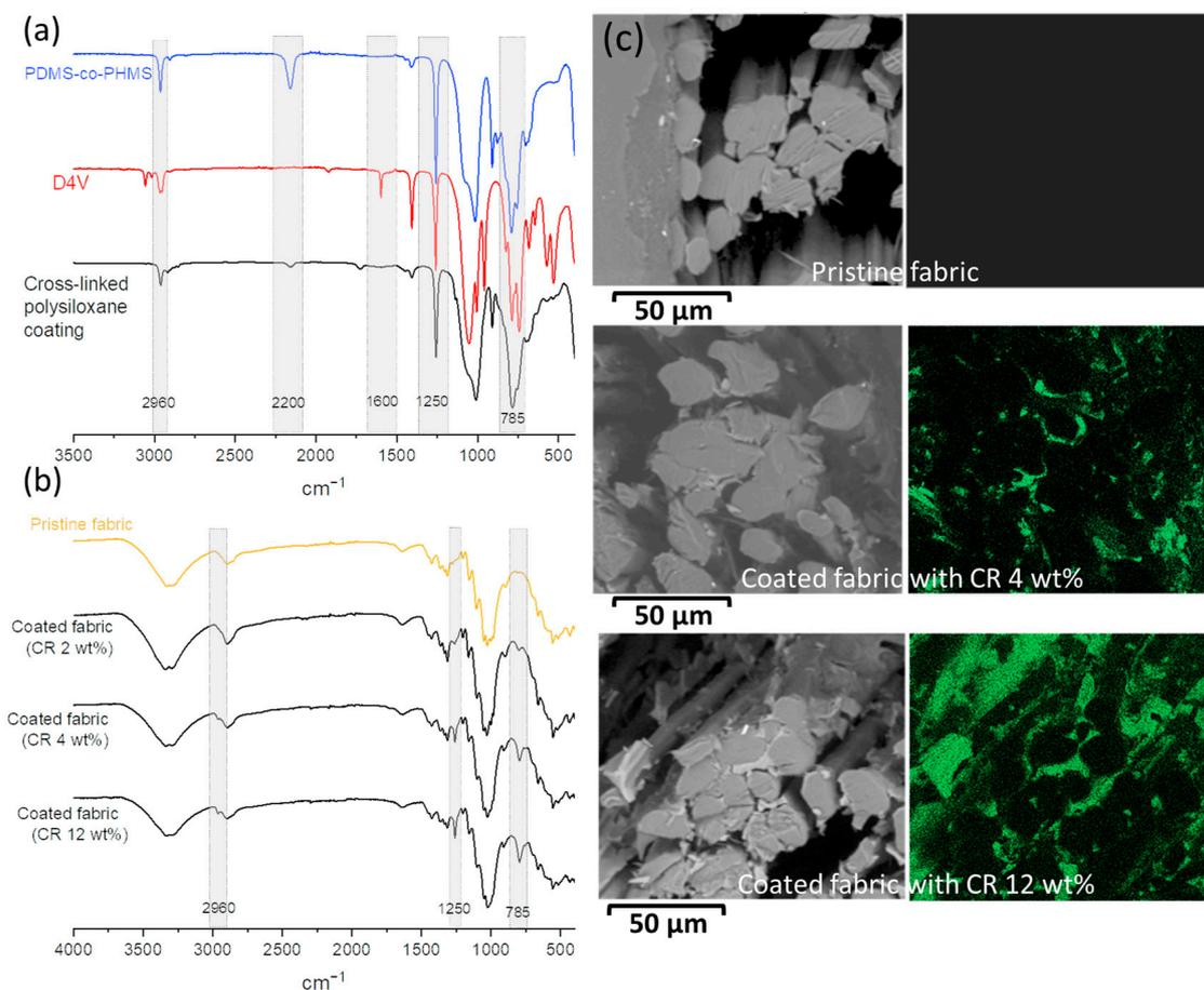
**Figure 3.** FTIR spectra for (a) PDMS-co-PHMS, D4V and the coating-based crosslinked polysiloxane. (b) Pristine and coated flax fabrics. (c) SEM/EDS images for pristine and coated fabrics of 4 and 12 wt% of CR.
