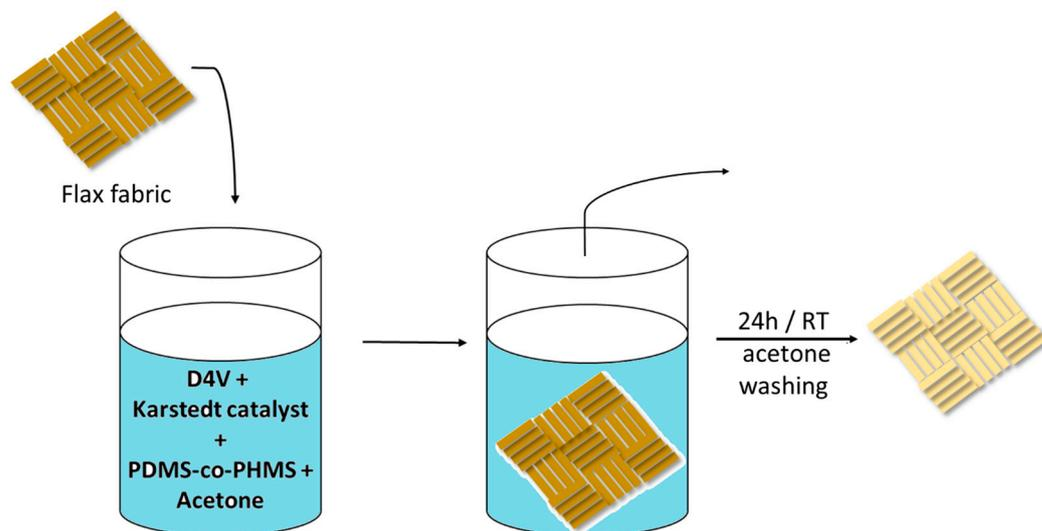
**Figure 7.** Scheme of the preparation of the hydrophobic flax fabrics via dip-coating method.
