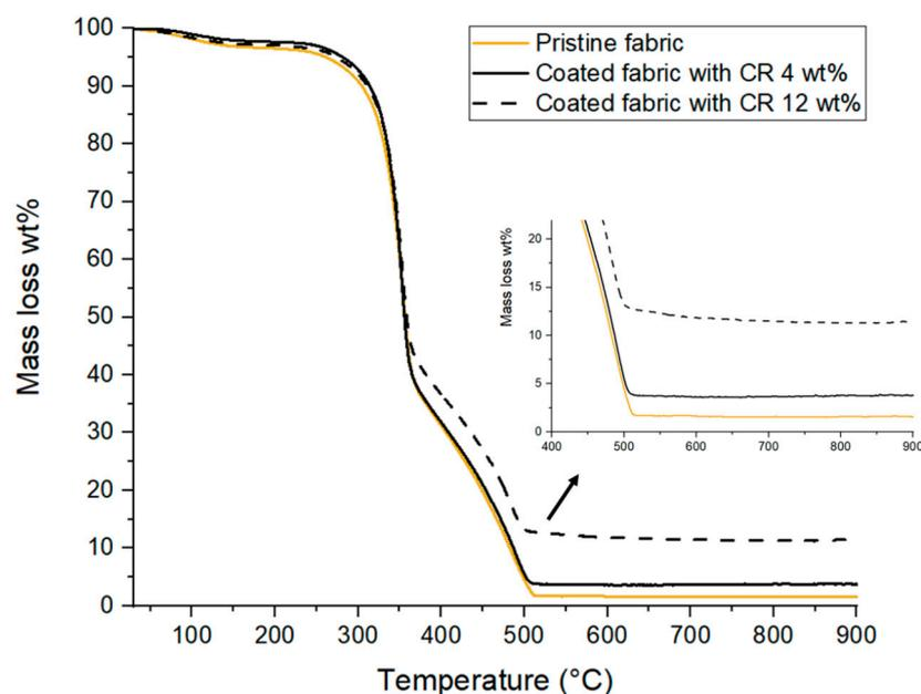
**Figure 2.** TGA curves of pristine and coated fabrics with 4 and 12 wt% of silicone.
