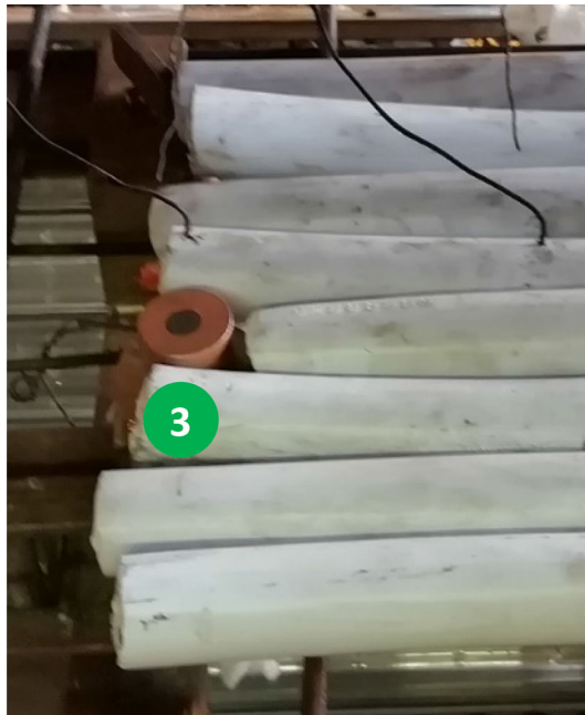
Figure 6. The Gardon water-cooled heat flux sensor (3) placed at the cable layer extremity.
