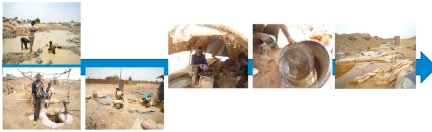
Fig. 2. ASM technical processes observed in the Liptako–Gourma region: From left to right: panning and extraction from wells, pre-treatment by crushing and sluice, amalgamation, and cyanidation (photo credits: Oumar Maman-Illatou).
