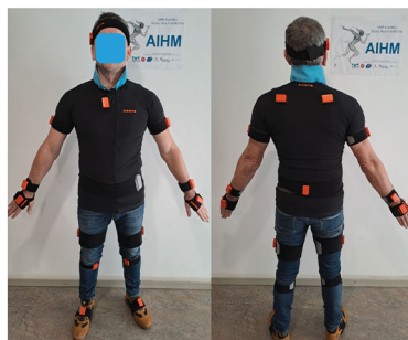
(a) M-Pose for location and placement of the full body inertial sensors using the guidelines set by XSens (placement for illustration only).
