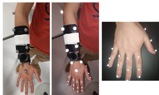
(b) Positioning of retro-reflective markers (10mm and 4mm in diameter, without and with flash) for studying the movements of the right arm.
