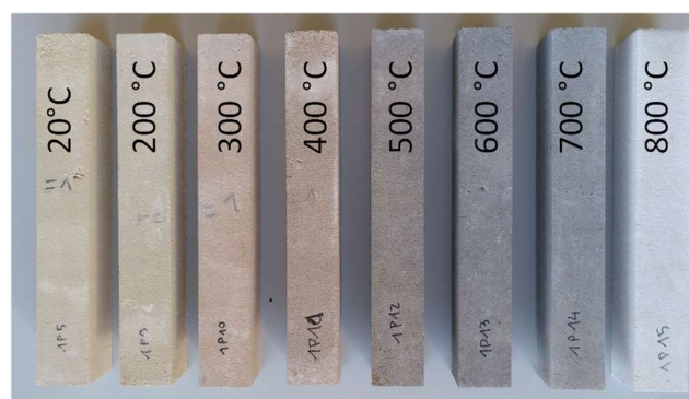
Fig. 2 Colour gradient of limestone 5 \times 5 \times 30 samples heated up to 800^\circ\text{C}
