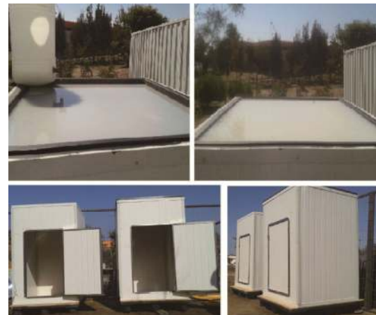
Fig. 3 Installation of test rooms with and without PCM
