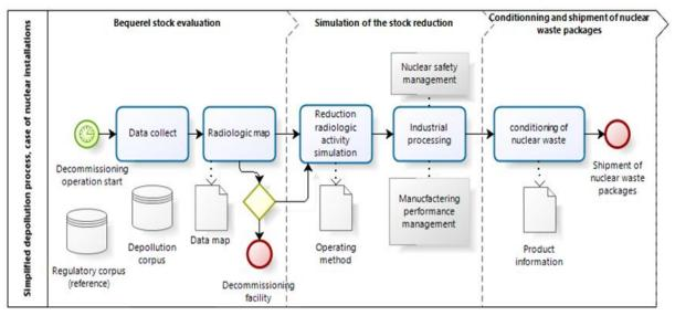
Figure 5: Simplified process of activity (Bq) reduction in three steps - nuclear facility dismantling
