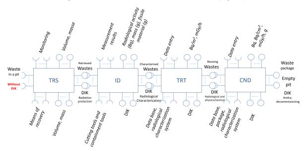
Figure 8: Proposition of an architecture for the treatment and conditioning of waste from a pit, inspired by Lessons Learned
