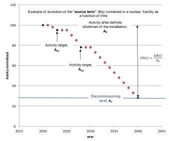
Figure 2: Reducing the source term by depollution operations - radiological contamination case
