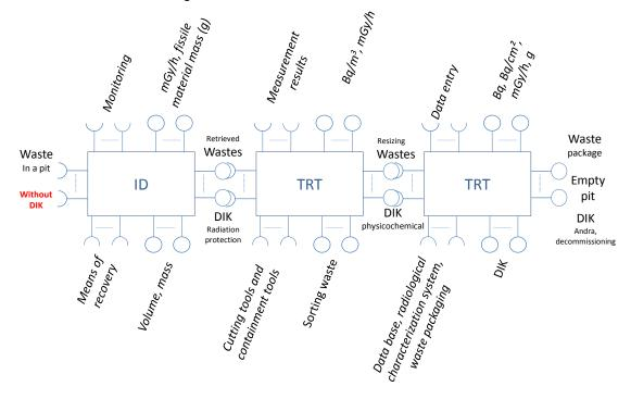
Figure 7: Proposition of an architecture for the treatment and conditioning of pit waste, with the data flux
