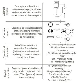
Figure 1: Ordinary Petri Nets DSML specification steps
