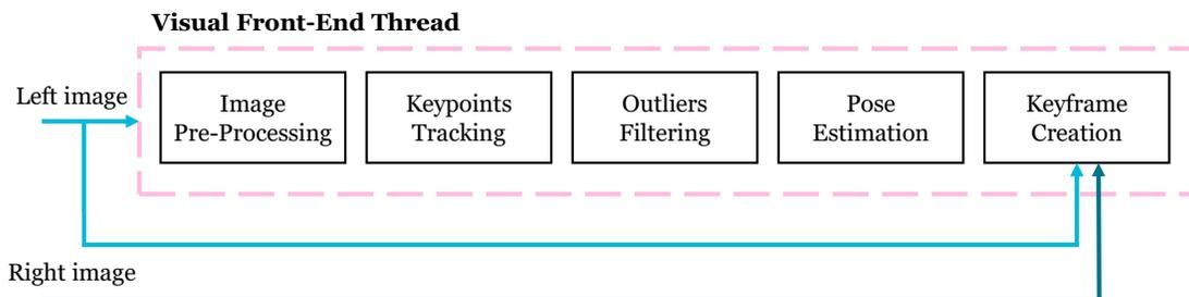
Fig. 3. Architecture of OV<sup>2</sup>SLAM with real-time processing presented in [4]. The front-end thread figured contain the corner detection methods. It is responsible for estimating the pose of the camera in real-time.
