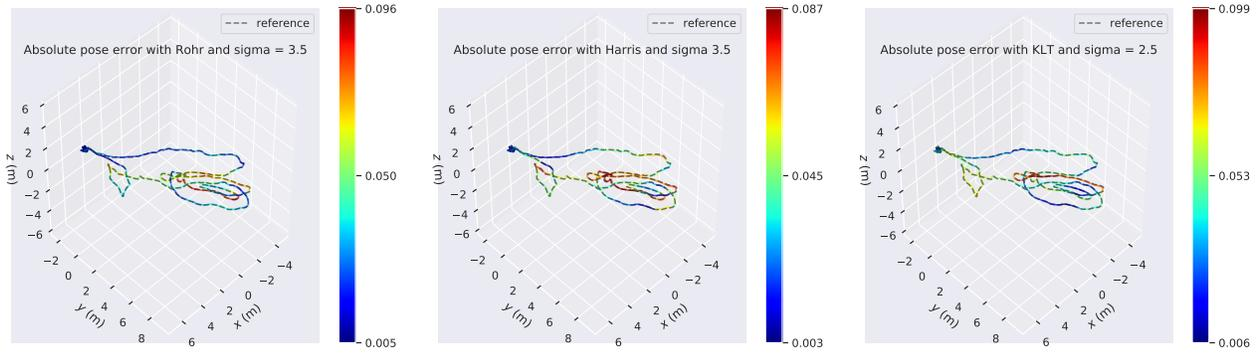
Fig. 4. 3D representation of the best path estimated by OV<sup>2</sup>SLAM with Rohr  $\sigma = 3, 5$  (left), Harris  $\sigma = 3, 5$  (center) and KLT  $\sigma = 2, 5$  (right). The represented path is tied to the Machine Hall 01 video containing 3682 stereo-pair images in all.
