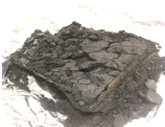
Fig. 1. Picture of the combustion residues after cone calorimeter of Sample 1 ( E + P + ENV ). It should be noticed that the top layer of the combustion residues of the envelope has been manually removed in order to make visible the combustion residues of the core material. The bottom layer of the combustion residues of the envelope is still visible.
