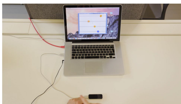
Figure 10. Display visible to the participant; the oscillatory movement of the preferred index finger was captured by a LEAP sensor (blue coded the moving circle of the participant in front of the screen and was always at bottom line of display, whilst the other moving circles of the other members of the same group were colour-coded as orange depicted in the upper lines of the display).
