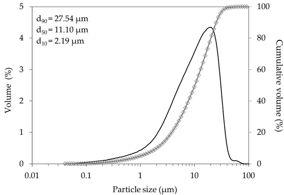
**Figure 1.** Particle size distribution of cement (Line: Volume (%); Line with diamonds: Cumulative volume (%)).
