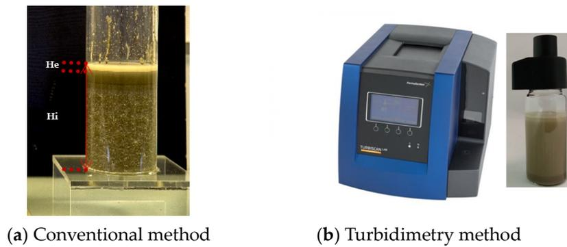
Figure 2. The apparatus used for the bleeding measurements.
