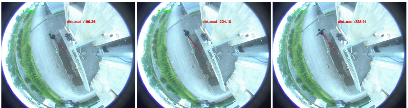
Fig. 10 Distance estimation approach between fisheye and target (1 m, 2 m and 3 m)
