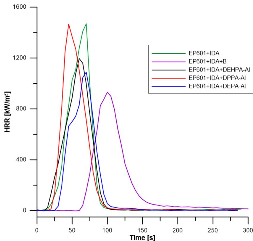
Figure 10. Cone calorimetry graphs for obtained composites.
