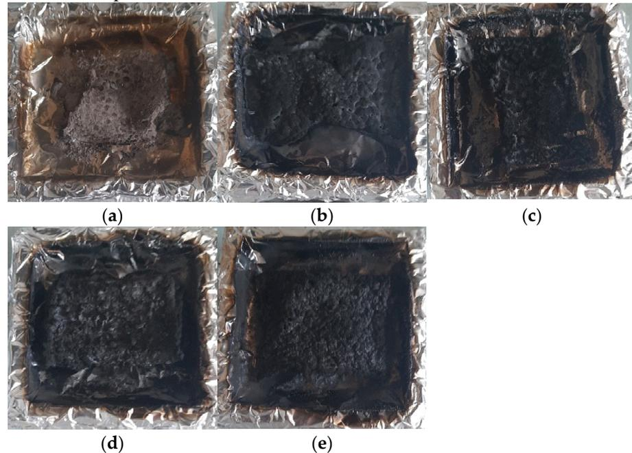
**Figure 11.** Photos of residue from cone calorimetry tests: (a) EP601 + IDA, (b) EP601 + IDA + B, (c) EP601 + IDA + DEHPA-Al, (d) EP601 + IDA + DPPA-Al, (e) EP601 + IDA + DEPA-Al.
