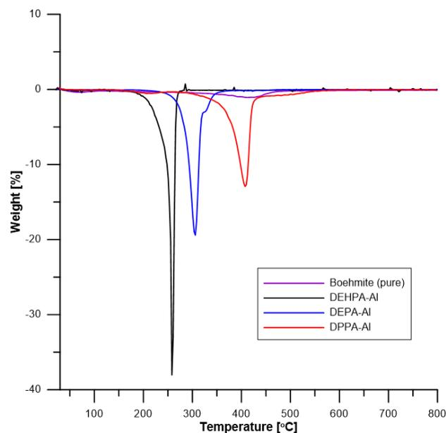
Figure 7. DTG curves of boehmite and hybrids (in helium).
