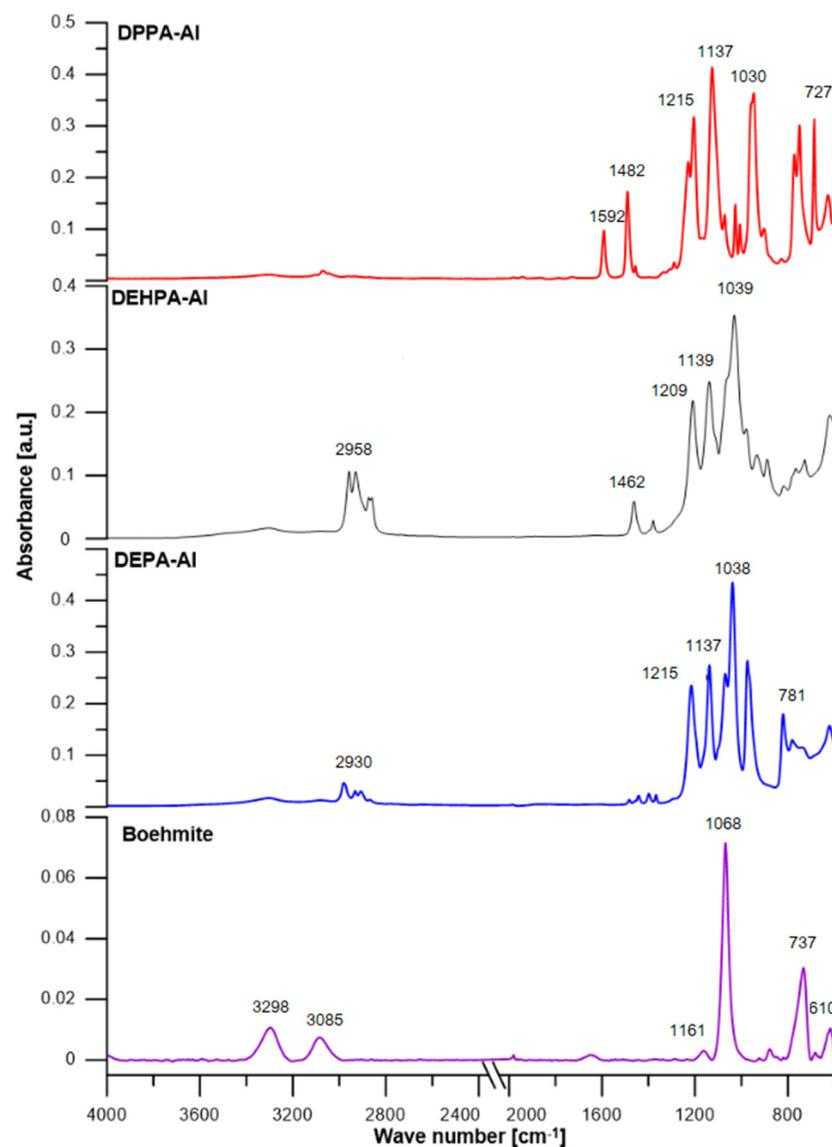
**Figure 4.** ATR-FT/IR spectra of boehmite and hybrids [ $\text{cm}^{-1}$ ].
