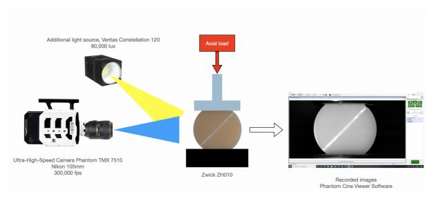
Figure 1. Scheme of the mechanical and optical setup.
