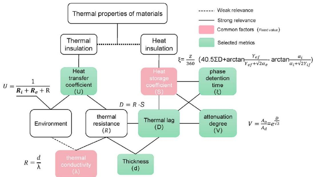
FIGURE 4. Relevance of the material's thermal parameters [15]
