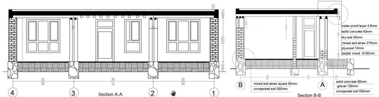
FIGURE 3. Prototype model, cross sections
