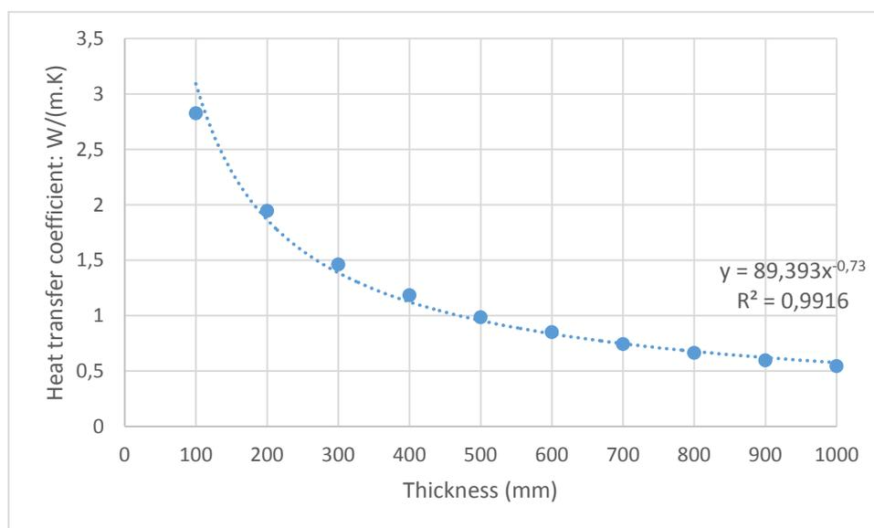
FIGURE 5. Fitting of the heat transfer coefficient
