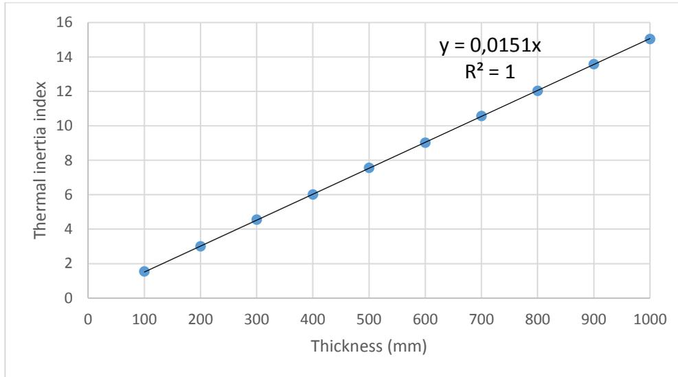
FIGURE 7. Thickness and thermal inertia index
