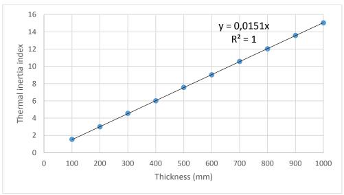
FIGURE 7. Thickness and thermal inertia index
