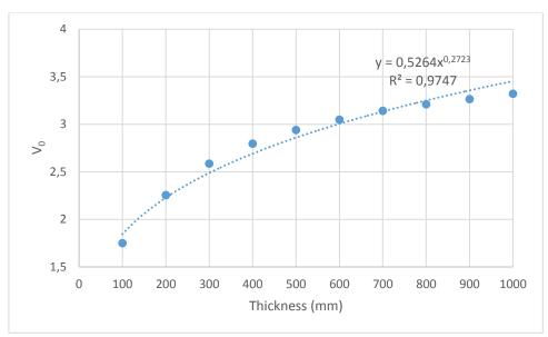
FIGURE 8. Fitting of the average annual attenuation of the temperature wave V<sub>0</sub>
