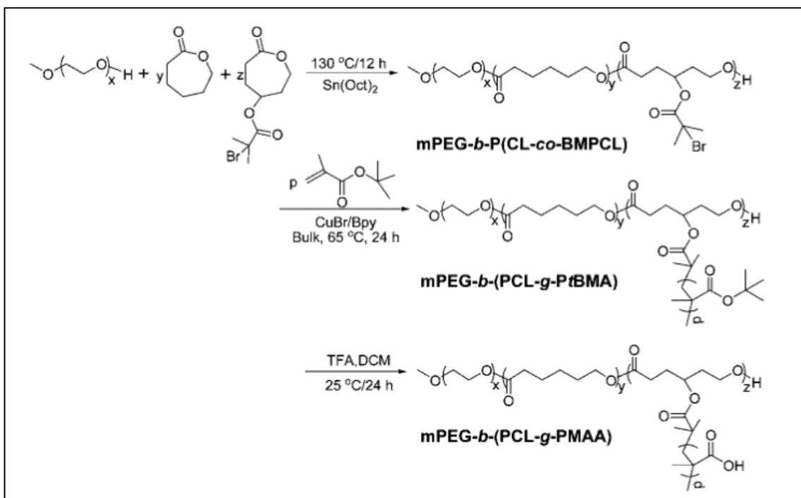
**Figure 10.** Synthesis routes of MeOPEG-*b*-(PCL-*g*-PMAA) (from Chang et al. [92]). Copyright Royal Society of Chemistry, reproduced with permission.
