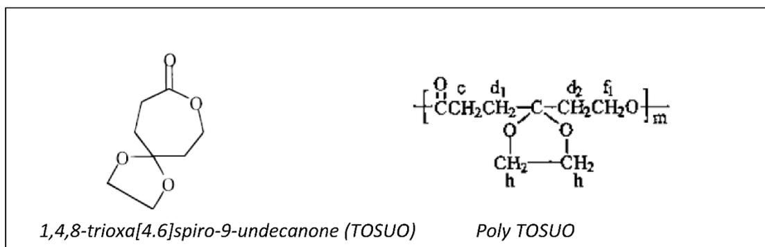
**Figure 20.** Structures of TOSUO and poly TOSUO.
