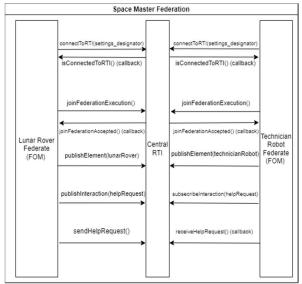
Fig. 3. HLA environment and methods used for communication
