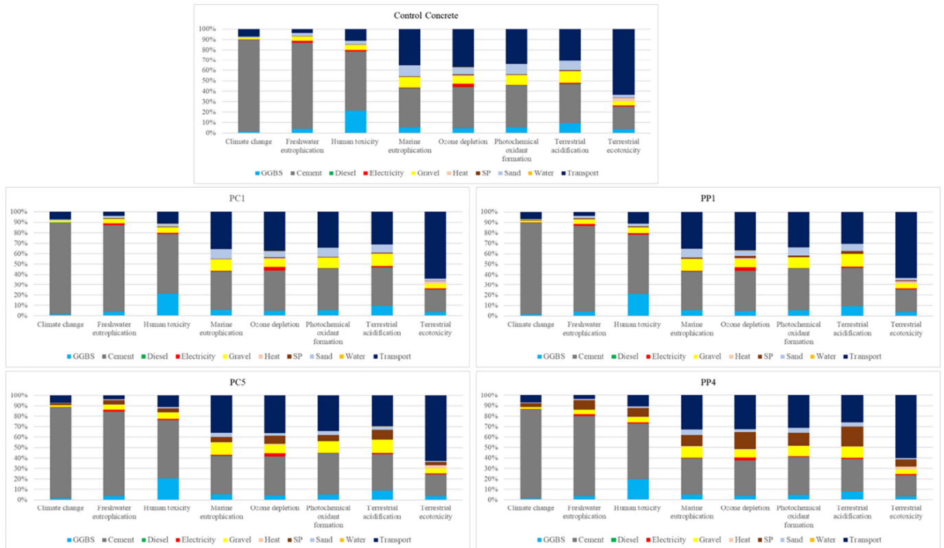
Fig. 5. Comparison of environmental impacts contributions between the extreme sand substitution by sediment within experimental concrete scenarios. Sand substitution by 10% sediment (PC1), 50% (PC5) and by 10% (PP1), 30% (PP4); PC: Port Camargue, PP: Port Perols.
