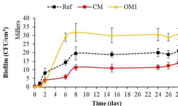
**Figure 1.** Quantification of bacterial colonization of mortar specimens. Each quantification was performed in triplicate using the culture-based method, and the error bars present the standard deviation from the values obtained. Ref = control mortar; CM = cured mortar; OM1 = oiled mortar prepared with CEM I.
