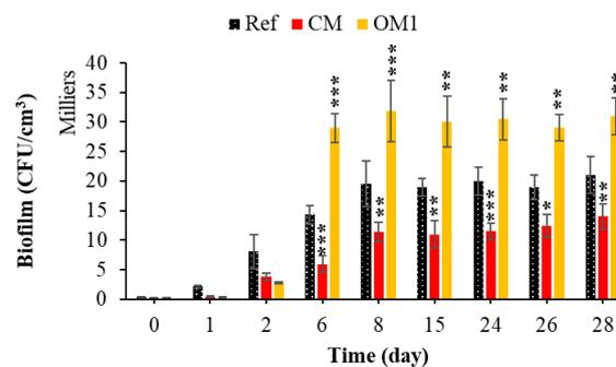
**Figure 2.** Statistical comparison (GraphPad Prism 5) of the biocolonization of mortar surfaces treated and untreated with curing compound or green formwork oil. Each experiment was performed in triplicate, and the error bars present the standard deviation of the values obtained. The experiments highlighted with asterisks differed significantly from the control (Bonferroni; \*\*:  $p < 0.01$ , \*\*\*:  $p < 0.001$ ) at the indicated time.
