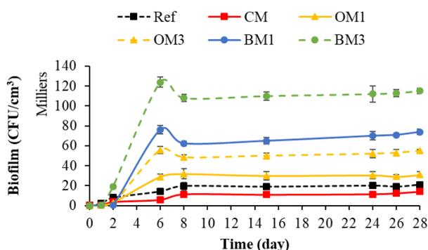
**Figure 3.** Quantification of bacterial-biofilm formation on mortar specimens. Each quantification was performed in triplicate using the culture-based method, and the error bars present the standard deviation from the values obtained. Ref = control mortar; CM = cured mortar; OM1 = oiled mortar prepared with CEM I; OM3 = oiled mortar prepared with CEM III; BM1 = biomimetic mortar prepared with CEM I; BM3 = biomimetic mortar prepared with CEM III.
