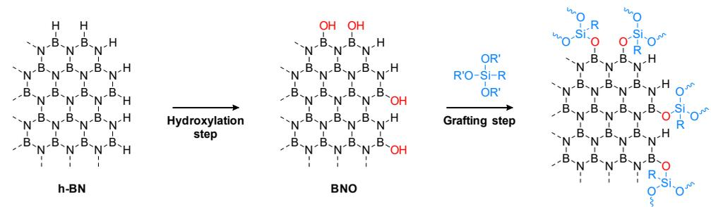
**Figure 2.** Schematic representation of the h-BN hydroxylation followed by a grafting step.
