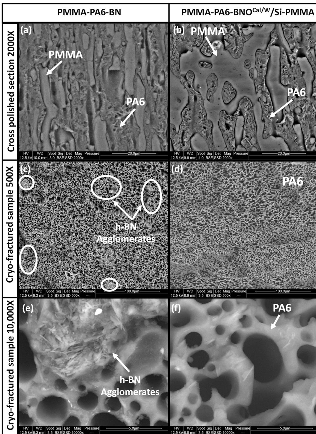
**Figure 13.** SEM images of PMMA-PA6-h-BN 8 wt% (left column) and PMMA-PA6-BNO<sup>Cal/W</sup>/Si-PMMA 8 wt% (right column). Parallel cross-polished sections (a,b) and perpendicular cryo-fractured surfaces after PMMA solvent extraction (c–f).
