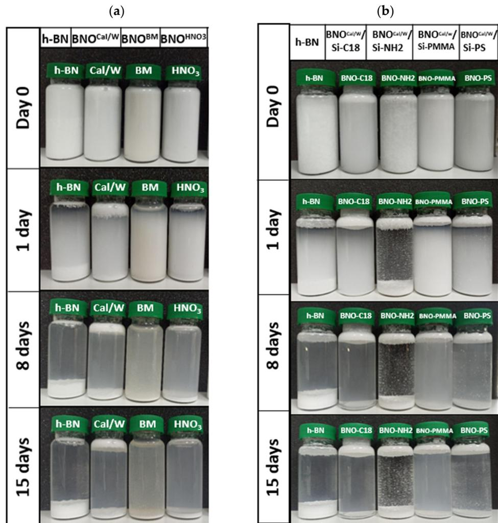
**Figure 5.** Photos of 0.6% wt suspensions in water. (a) Hydroxylated h-BN and (b) grafted BNO<sup>Cal</sup>.
