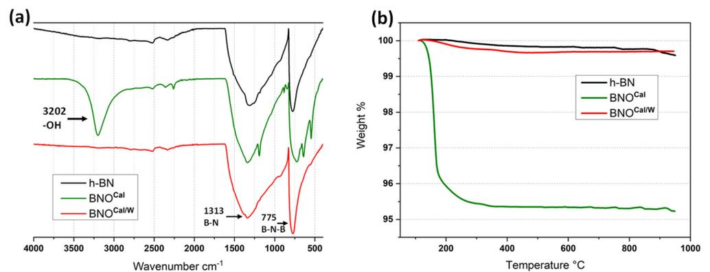
**Figure 3.** FTIR spectra (a) and TGA thermograms (b) of h-BN, BNO<sup>Cal</sup>, and BNO<sup>Cal/W</sup> samples.
