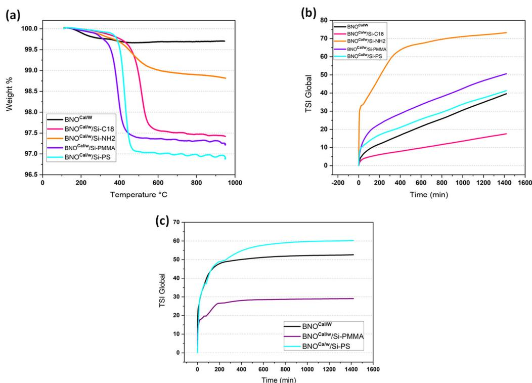
**Figure 11.** (a) TGA of grafted  $\text{BNO}^{\text{Cal/W}}$  compared with that of  $\text{BNO}^{\text{Cal/W}}$ . (b) TSI global in water and (c) TSI global in toluene for  $\text{BNO}^{\text{Cal/W}}$  and grafted  $\text{BNO}^{\text{Cal/W}}$ .
