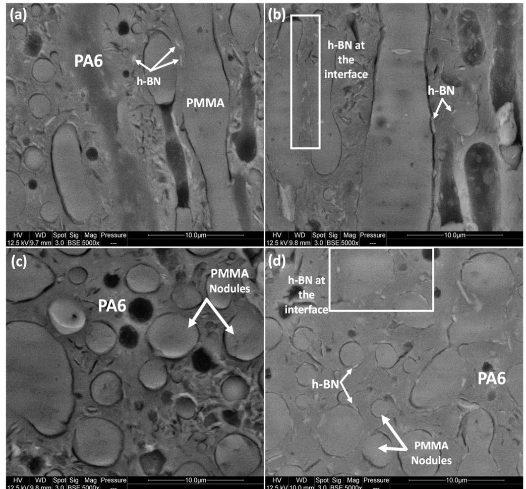
**Figure 14.** SEM images of (PMMA+h-BN)-PA6 with 8 wt% of h-BN (left column) and (PMMA +  $\text{BNO}^{\text{Cal/W}}/\text{Si-PMMA}$ )-PA6 with 8 wt% of  $\text{BNO}^{\text{Cal/W}}/\text{Si-PMMA}$  (right column). Parallel cross-polished sections (a,c) and perpendicular cryo-fractured surfaces (b,d).
