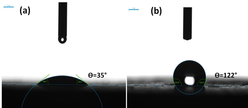
**Figure 12.** Water drop shape at the surface of (a) h-BN and (b) BNO<sup>Cal/W</sup>/Si-PMMA.
