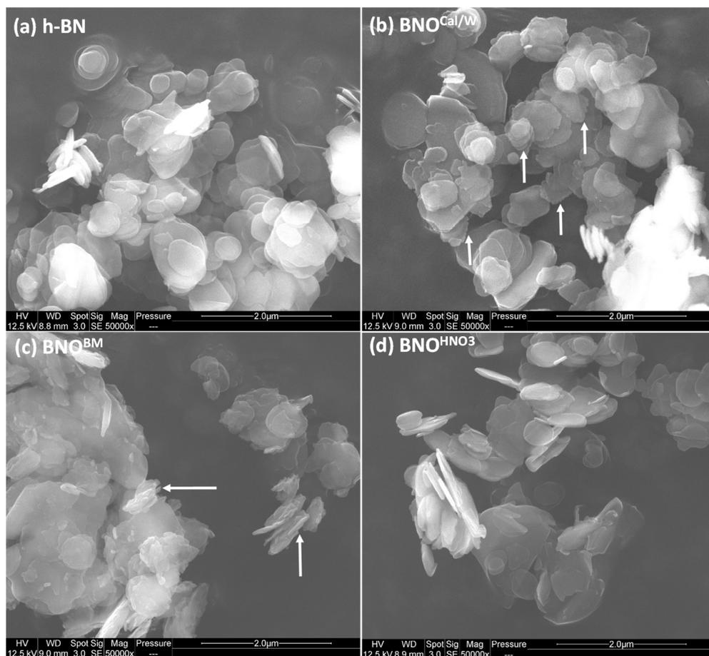
**Figure 7.** SEM images of (a) h-BN, (b)  $\text{BNO}^{\text{Cal/W}}$ , (c)  $\text{BNO}^{\text{BM}}$ , and (d)  $\text{BNO}^{\text{HNO}_3}$  samples. Magnification: 50,000 $\times$ , scale bar = 2  $\mu\text{m}$ , and arrows indicate the evolution of the edges of the sheets.
