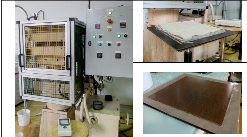
Figure 1. Manufacturing of the Flax fibre biocomposites using thermopress
