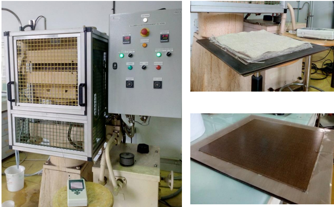
Figure 1. Manufacturing of the Flax-PP composite using thermopress
