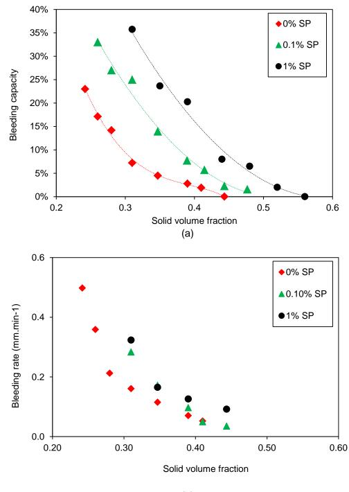
(b) Fig. 5. Bleeding capacity (a) and bleeding rate (b) as a function of solid volume fraction 460
