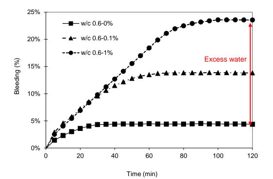
Fig. 6. Evolution of bleeding for cement pastes with time for w/c ratio of 0.6 (solid volume fraction of 0.35)
