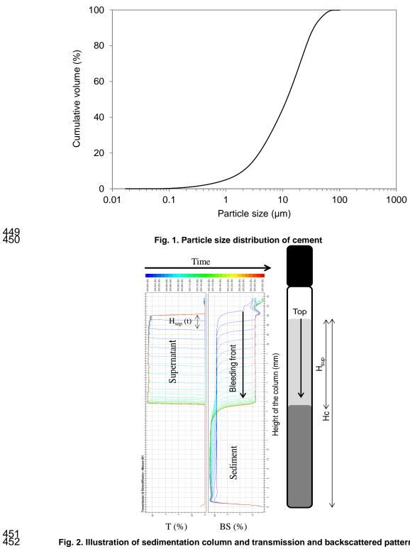
Fig. 2. Illustration of sedimentation column and transmission and backscattered patterns
