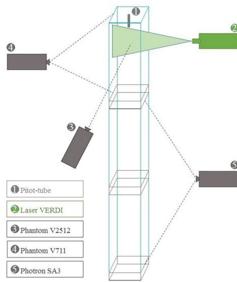
Figure 1: Schema of configuration for measuring propagation velocity and unburned flow velocity
