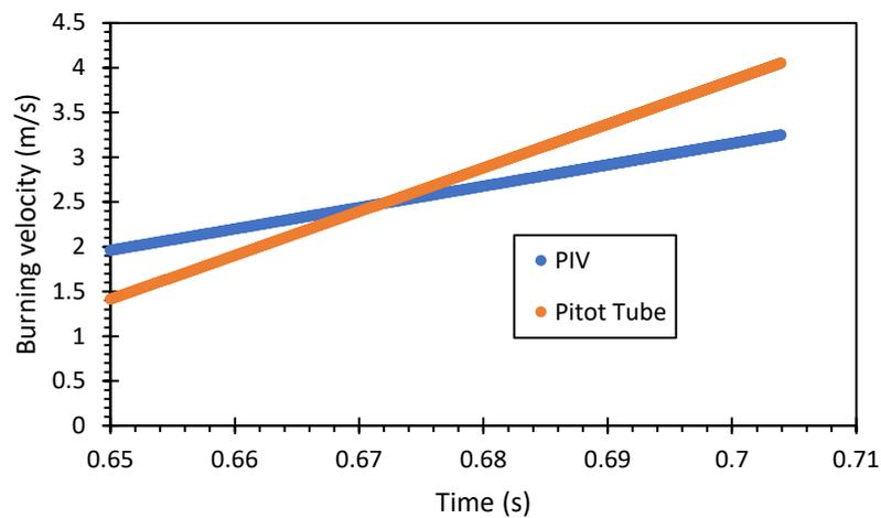
Figure 6: Evolution of burning velocity. Comparison of PIV and Pitot tube results
