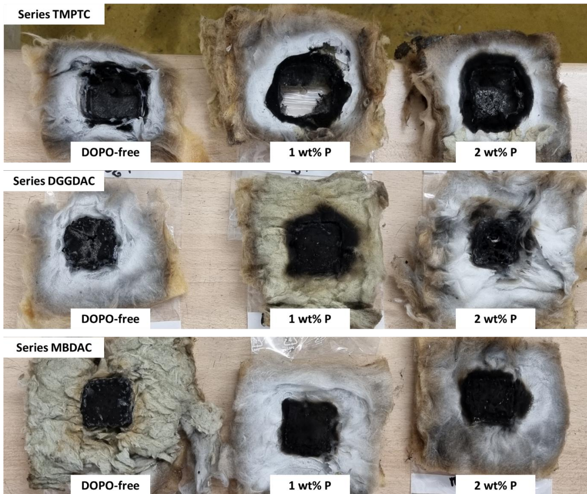
Figure 22: Residues of the foams after cone calorimeter test
