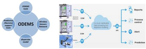
Figure 1. ODEMS principle and structure
