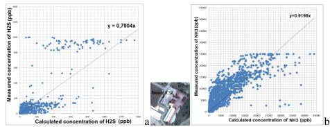
Figure 7: correlation between measured and calculated value on sensor  $n^{\circ}12$  (a) H2S (b)NH3
