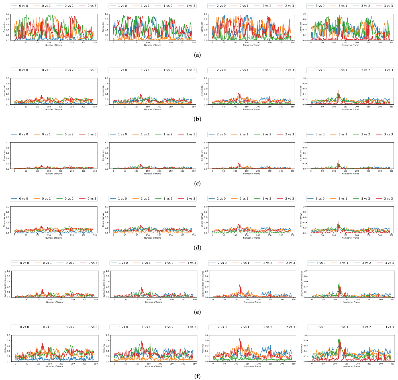
Figure 8. Curves comparing persons from one frame to another in video 1 (persons 0, 1, 2, and 3) using the HOG. (a) Correlation. (b) Intersection. (c) Chi-square. (d) Bhattacharyya. (e) KL divergence. (f) Minkowski.
