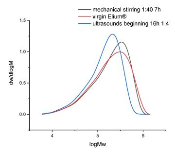
Figure 14. Molecular weights distribution of virgin Elium<sup>®</sup> and recycled Elium<sup>®</sup> resin after dissolution.
