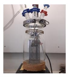
Figure 1. Experimental device used for dissolution experiments using mechanical stirring.
