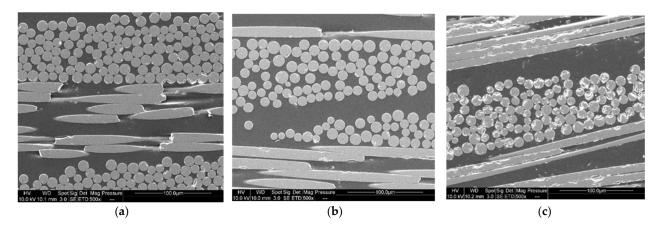
**Figure 15.** SEM images of (**a**) first generation composite (**b**) second generation composite after dissolution using mechanical stirring and (**c**) second generation composite after dissolution using ultrasound in the beginning.
