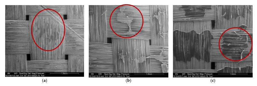
**Figure 10.** SEM image of (**a**) Basalt fibers recovered by mechanical stirring (1:40 ratio) during 7 h, (**b**) Basalt fibers recovered with ultrasound at the beginning of the dissolution (1:4 ratio) during 16 h and (**c**) Basalt fibers recovered with ultrasound at the end of the dissolution (1:4 ratio) during 7 h.
