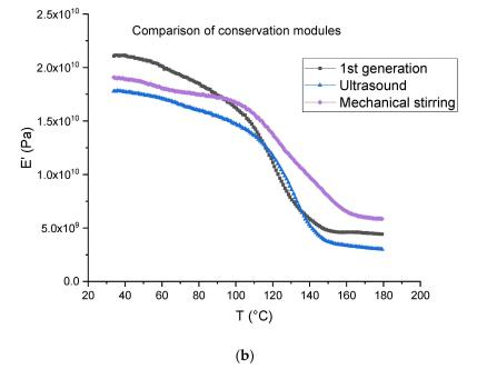
**Figure 16.** (a) Tangent delta; (b) conservation modulus of first-generation composites and second-generation composites obtained after dissolution using mechanical stirring and ultrasounds.
