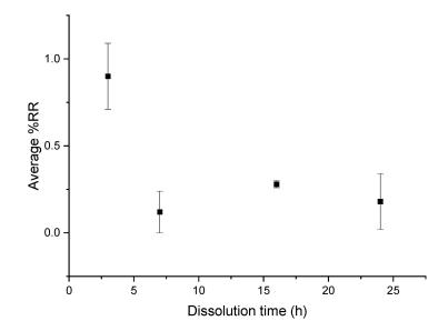
**Figure 12.** Evolution of the average %*RR* as a function of time for recycling with mechanical stirring and acetone at a ratio of 1:40.
