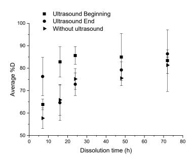
**Figure 3.** Influence of different ultrasonic conditions on the average %*D* as a function of dissolution time for a "composite:acetone" ratio of 1:4.
