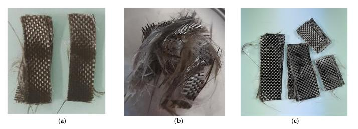
**Figure 5.** Basalt fibers recovered (**a**) after recycling 16 h with ultrasound at the beginning of the dissolution, (**b**) after recycling 7 h with ultrasounds at the end of the dissolution and (**c**) after recycling without ultrasounds. A 1:4 ratio is considered for each photo.
