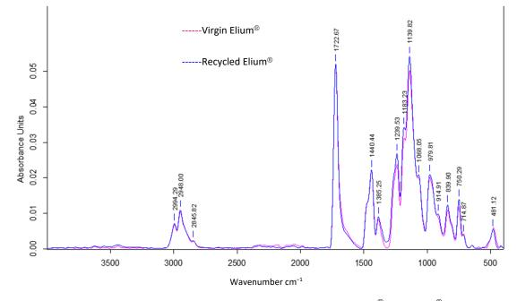
**Figure 13.** ATR FTIR absorbance spectrum of virgin Elium<sup>®</sup> and Elium<sup>®</sup> after 24 h of simple dissolution in acetone 1:4.
