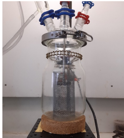
Figure 1. Experimental device used for dissolution experiments using mechanical stirring.
