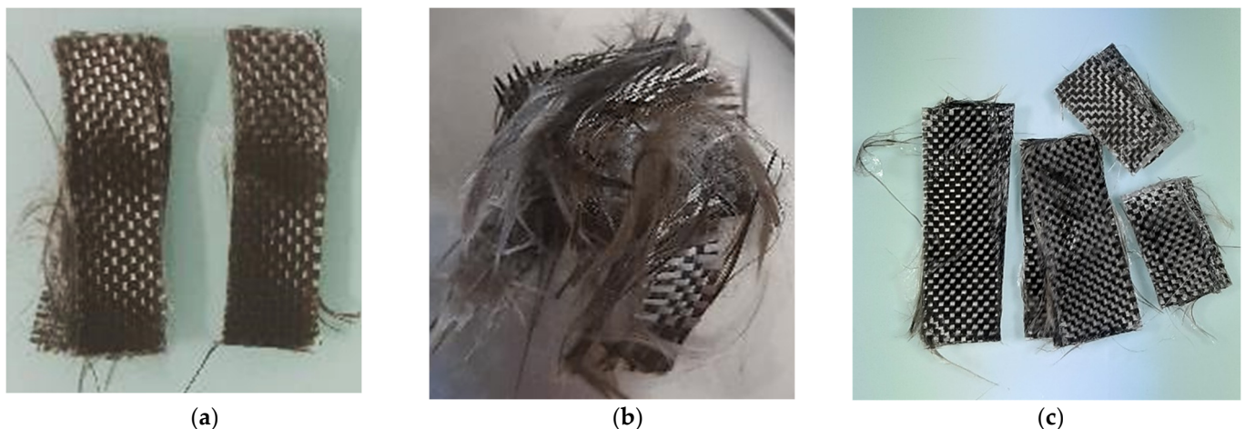
Figure 5. Basalt fibers recovered (a) after recycling 16 h with ultrasound at the beginning of the dissolution, (b) after recycling 7 h with ultrasounds at the end of the dissolution and (c) after recycling without ultrasounds. A 1:4 ratio is considered for each photo.
