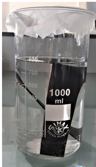
Figure 2. Experimental device used for dissolution experiments using ultrasounds.
