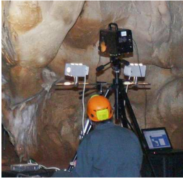
Figure 3: View of the spectroradiometer and light sources used in situ .
