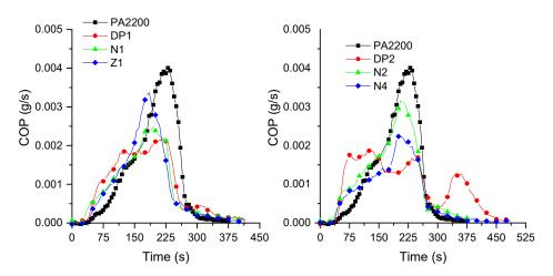
Figure 5. CO production of PA12 and PA12/NBR blends.
