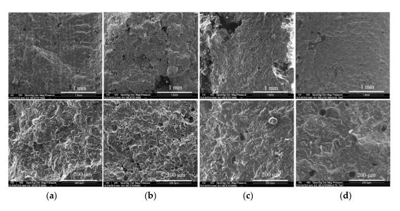
Figure 2. SEM images of LS printed parts at 100 and 500×: (a) PA2200; (b) DP2; (c) N2; and (d) Z2.
