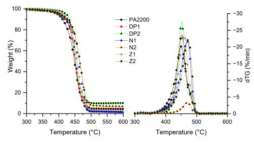
Figure 3. Mass loss curves of formulations under nitrogen at 10 °C/min.
