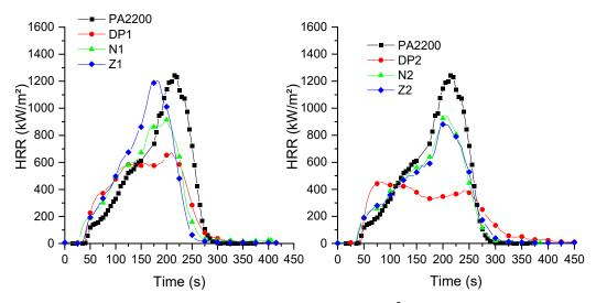
Figure 4. Heat release rates of compositions (irradiance: 50 kW/m<sup>2</sup>).
