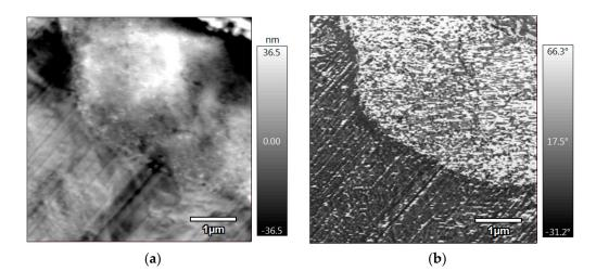
Figure 9. (a) AFM topography, and (b) phase images of DP2 formulation.
