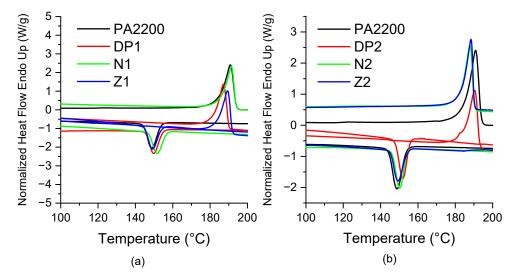
Figure 1. Thermograms of (a) formulations containing 10wt.% and (b) 20wt.% blends.
