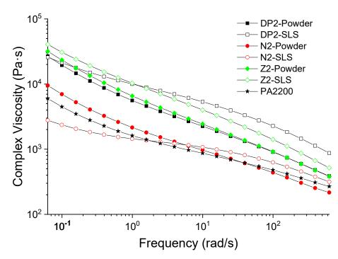
**Figure 7.** Complex viscosities of PA12 and PA12/NBR blends at 210 °C as a function of angular velocity. Unfilled symbols: LS samples; filled symbols: thermocompressed samples.
