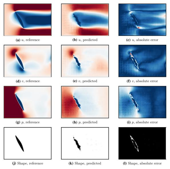
Fig. 17 Flow and shape predictions around an enlarged Bezier shape. As this input shape is an outlier, the shape reconstruction is poor, and is associated with large prediction errors ( $e_f = 1.316 \times 10^{-2}$ ). For the u, v and p predictions, the color scales are the same as for Fig. 4
