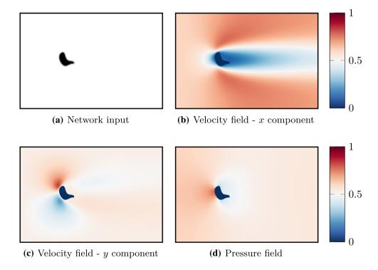
each block in the decoder branches. Finally, a convolutional layer with a  $1 \times 1$  kernel is applied to set the final number of channels (1 for the shape decoder, and 3 for the flow decoder). The output of our network hence contains 1-channel tensor representing reconstructed input, and a 3-channel tensor representing the velocity and pressure.
