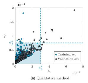
**Fig. 6** Description of the qualitative and quantitative methods on the scatter plots of  $e_f$  versus  $e_s$  on training and validation sets for a reference twin-decoder architecture. (Left) Qualitative method: given a threshold  $e_f^*$ , the corresponding optimal  $e_s^*$  is found by solving problem (6). Then, the end-user rejects predictions that produce shape reconstruction errors superior to  $e_s^*$ . Only the predictions falling
