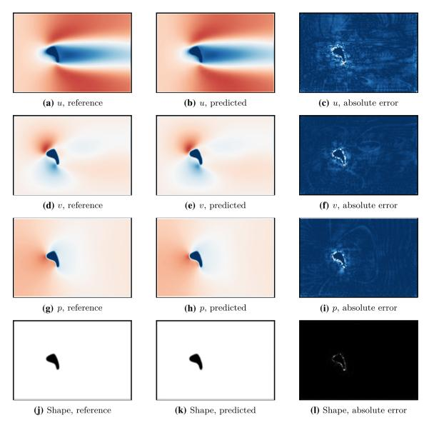
**Fig. 9** Flow and shape predictions around an obstacle from the test set. On this instance, the flow prediction error is  $e_f = 1.57 \times 10^{-5}$ , with most of the error concentrated on the boundary of the shape,
