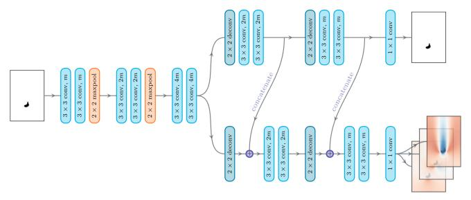
**Fig. 5** Proposed twin-decoder architecture. The encoder is based on a pattern made of two convolutional layers followed by a max-pooling layer. At each occurrence of the pattern, the image size is divided by two, while the number of filters, noted m, is doubled. In both decoder paths, a transposed convolution step is first applied to the input, while the number of filters is halved. The output of this layer in the flow
