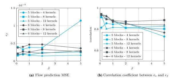
Fig. 7 Hyper-parameter calibration. The performance is evaluated on the validation set. To compare the accuracy of flow prediction between different architectures, the MSE is averaged over the entire dataset
