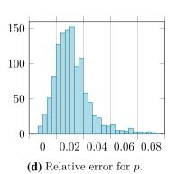
Fig. 10 Relative error for flow predictions over test set. The black rectangle around the obstacle indicates the area on which the u, v and p relative errors are computed. The histograms indicate the error levels obtained when comparing predictions to labels on the 1200 elements of the test set
