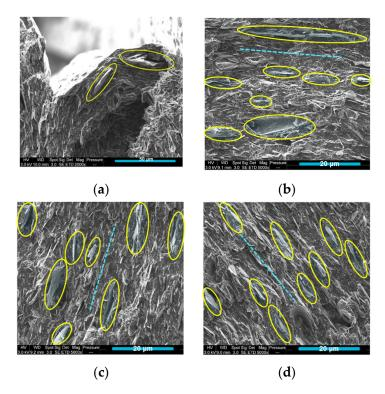
**Figure 8.** (a) SEM image of 3D-printed PLA/PCL/15 wt% M5; (b-d) SEM images of injection-moulded PLA/PCL/15 wt.% M5 composite (The yellow ellipses are surround some graphene flakes and the dotted lines indicate the similar orientation of the graphene platelets in the injection moulded samples).
