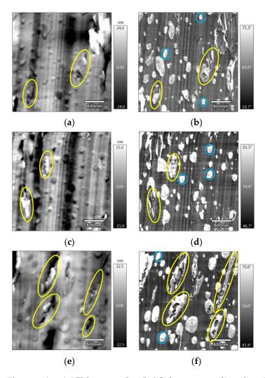
**Figure 5.** (a,c,e) AFM topography; (b,d,f) the corresponding phase images of (a,c,e), respectively, of the injection-moulded PLA/PCL/10 wt.% M5 (the yellow circles surround the PCL particles containing GNPs and the blue circles surround the pure PCL nodules).
