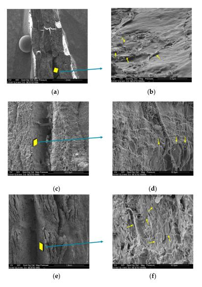
**Figure 10.** (**a**,**c**,**e**) SEM images at the interface of two 3D printed filaments of PLA/PCL/15 wt.% M5 composites; (**b**,**d**,**f**) the zoomed images of (**a**,**c**,**e**), respectively (the yellow arrows are pointed towards some graphene nanoplatelets).
