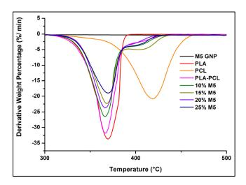
**Figure 13.** DTG curves (N2 atmosphere,  $10 \, ^{\circ}$ C.min<sup>-1</sup>) of GNP, PLA, PCL, and PLA/PCL blends and their composites.
