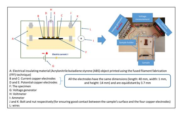
Figure 2. The setup of the electrical resistance measurement using the four probes method.
