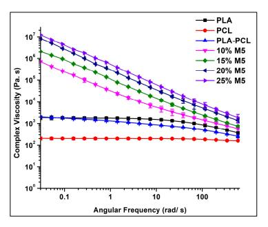
**Figure 12.** The complex viscosity curves of pure PLA and PCL polymers in addition to their blend and composites.
