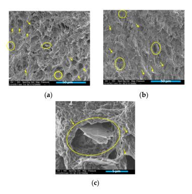
**Figure 7.** (**a**,**c**) SEM images of toluene-etched, injection-moulded PLA/PCL/10 wt.% M5 composite; (**b**) SEM images of toluene-etched, 3D-printed PLA/PCL/10 wt.% M5 composite (The yellow circles surround the GNPs positioned in the pores where the PCL nodules were expected to be located and the yellow fleshes are pointed towards these pores).
