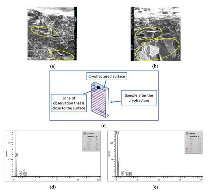
**Figure 9.** (a) SEM image of the injection-moulded PLA/PCL/15 wt.% M5 composite and its EDX (d); (b) SEM image of 3D printed PLA/PCL/15 wt.% M5 composite and its EDX (e); (c) the zone of observation where (a,b) were determined and indicated by the small black circle (the yellow circles surround some graphene flakes).
