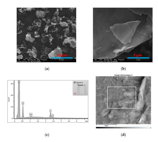
**Figure 3.** (a,b) SEM images of M5 GNP at different magnifications; (c) EDX graph; (d) the part of the surface that is surrounded by a rectangle and whose surface elements are shown in the EDX graph (c).
