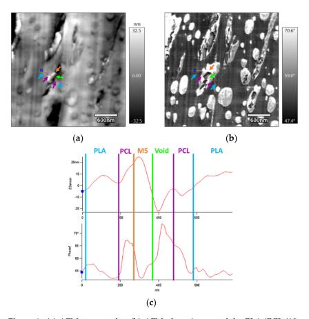
**Figure 4.** (a) AFM topography; (b) AFM phase images of the PLA/PCL/10 wt.% M5 injection-moulded sample; (c) topography and phase profiles on a drawn red line that is traced in (a,b) (the fleshes in the images point towards the different components of the composite and their colours match the designation of the peaks in the profiles).
