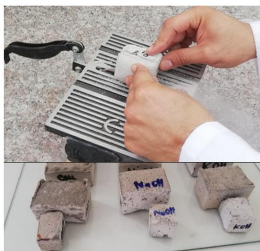
Figure 11. The ease of cutting the prepared insulating geopolymers with a circular saw.
