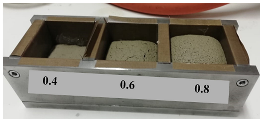
Figure 6. Progressive swelling of the samples with an increase in the water/ash ratio (0.4, 0.6 and 0.8).
