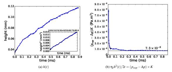
Figure 4: Capillary rise in a random structure : average position of the flow front over time (a) and corresponding values  $p_{cap}K$  (b).
