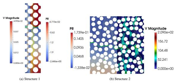
Figure 2: Capillary rise in hexagonal (structure 1) and random (structure 2) structures: flow front, pressure, velocity intensity and streamlines.
