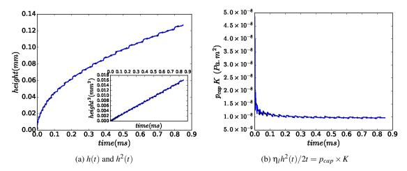
Figure 3: Capillary rise in a hexagonal structure: average position of the flow front over time (a) and corresponding values of  $p_{cap}K$  (b).
