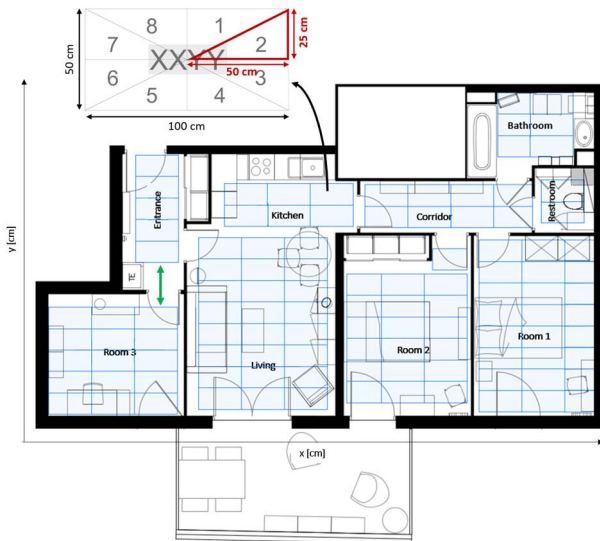
Fig. 1. Map of the apartment with furniture, sectors arrangement and gaps (green). Each sector is composed of 8 sensors (Insert in red). Gaps are “empty” locations, not equipped with sensors, and are mainly found between rooms or under fixed pieces of furniture. Some sectors were cut during installation.
