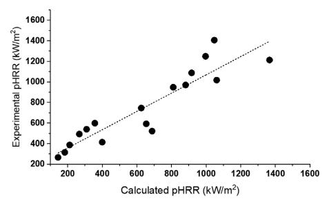
Fig. 2. Relationships between experimental pHRR measured at 50 kW/m<sup>2</sup> versus calculated pHRR.
