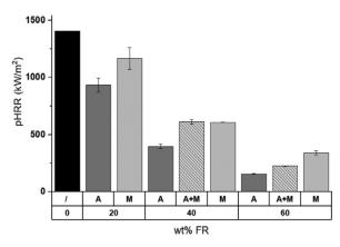
**Fig. 4.** pHRR in cone calorimetry (50 kW/m<sup>2</sup>) for EVA-PE filled with ATH (A), MDH (M) and ATH+MDH (A + M).
