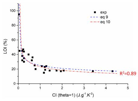
Fig. 1. LOI versus calculated index: experimental data and Eqs. (9) and (10).
