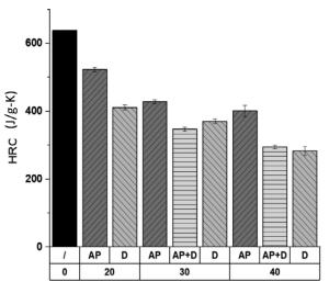
Fig. 8. HRC measured by PCFC for ABS filled with APP and DBDPO.
