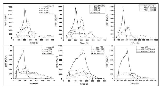
Fig. 3. Cone calorimeter curves for flame retarded EVA/PE and ABS at 50 kW/m<sup>2</sup>.
