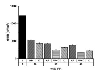
**Fig. 5.** pHRR in cone calorimetry (50 kW/m<sup>2</sup>) for ABS filled with APP (AP), DBDPO (D) and APP+DBDPO (AP+D).
