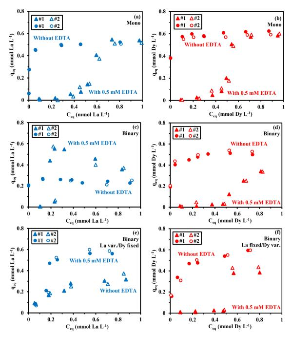
**Fig. 3.** La(III) (a, c, and e) and Dy(III) (b, d, and f) sorption isotherms at  $pH_0$  6 in presence and absence of EDTA (0.5 mM) for mono-component solutions (a and b), binary equimolar solutions (c and d), and binary solutions with variable La/Dy molar ratio (fixed D(III) concentration and variable La(III) concentration, and reciprocal; e and f).(SD: 0.5 g L<sup>-1</sup>; contat time: 48 h; T: 20  $\pm$  1 °C; duplicate series: #1 and #2).
