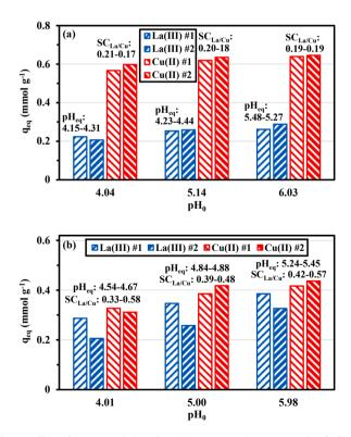
**Fig. 8.** Effect of pH<sub>0</sub> on La(III) and Cu(II) sorption using AO-APEI beads from bi-component solutions in the absence (a) and in the presence (b) of EDTA (C<sub>0</sub> (metal): 0.5 mmol L<sup>-1</sup>; EDTA concentration: 0.5 mmol L<sup>-1</sup> (when relevant); time: 48 h; SD: 0.5 g L<sup>-1</sup>; additional information: equilibrium pH and SC<sub>La/Cu</sub> values; duplicate series: #1 and #2).
