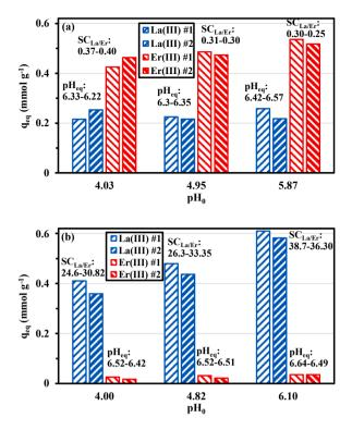
**Fig. 7.** Effect of pH<sub>0</sub> on La(III) and Er(III) sorption using AO-APEI beads from bi-component solutions in the absence (a) and in the presence (b) of EDTA ( $C_0$  (metal): 0.5 mmol L<sup>-1</sup>; EDTA concentration: 0.5 mmol L<sup>-1</sup> (when relevant); time: 48 h; SD: 0.5 g L<sup>-1</sup>; additional information: equilibrium pH and SC<sub>La/Er</sub> values; duplicate series: #1 and #2).
