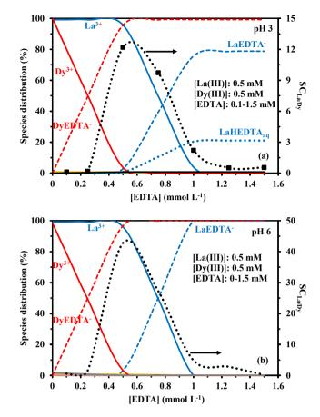
**Fig. 6.** Correlation between the SC<sub>La/Dy</sub> and La(III)-Dy(III) speciation diagrams at pH 3 (a) and pH 6 (b) for increasing concentrations of EDTA ( $C_0$ : 0.5 mmol L<sup>-1</sup>; example of correlation with Series #1 from Fig. 5).
