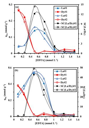
Fig. 5. Effect of EDTA concentration on La(III) and Dy(III) sorption capacities from binary equimolar solutions (C<sub>0</sub>: 0.5 mmol  $L^{-1}$ ) and SC<sub>La/Dy</sub> at pH<sub>0</sub> 3 (a) and pH<sub>0</sub> 6 (b).
