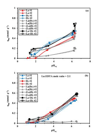
**Fig. 1.** Effect of pH on La(III) and Dy(III) sorption using AO-APEI beads from mono- and bi-component solutions in the absence (a) and in the presence (b) of EDTA ( $C_0$  (metal): 0.5 mmol L<sup>-1</sup>; EDTA concentration: 0.25 mmol L<sup>-1</sup> for monometal solutions and 0.5 mmol L<sup>-1</sup> for binary solutions (when relevant); time: 48 h; SD: 0.5 g L<sup>-1</sup>; duplicate series: #1 and #2; La + Dy, corresponds to cumulative sorption capacities for binary solutions).
