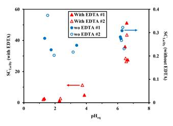
**Fig. 2.** Effect of the pH and the presence of EDTA on the selectivity of La/Dy sorption using AO-APEI beads ( $C_0$ : 0.5 mmol L<sup>-1</sup>; EDTA concentration: 0.5 mmol L<sup>-1</sup> (when relevant); time: 48 h; SD: 0.5 g L<sup>-1</sup>; duplicate series: #1 and #2).
