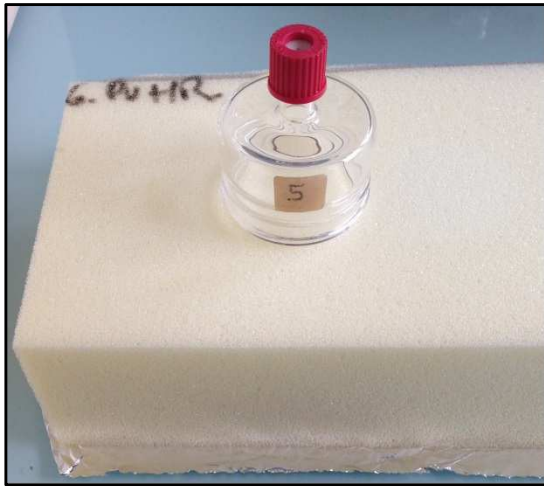
Figure 1. Pictures showing the emission cell placed on the material surface before sampling (a) and SVOCs sampling by SPME in the cell (b).
