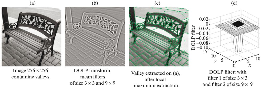
Fig. 3. Valley detection using a DOLP filter.
