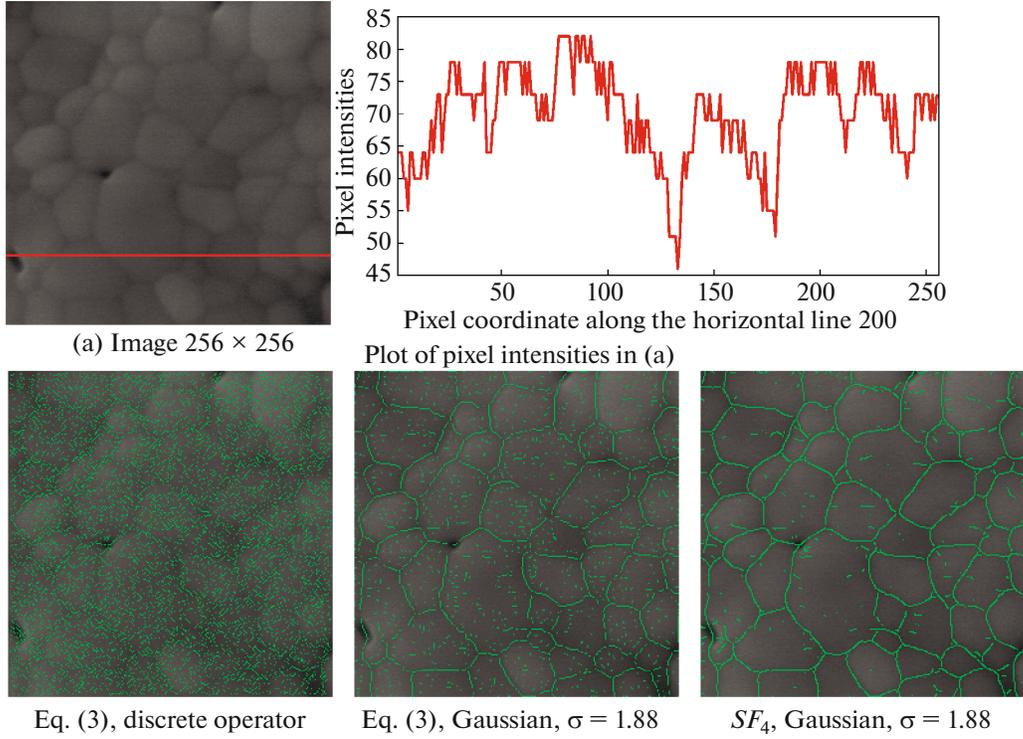
**Fig. 7.** Comparison of valley detection on real images. The image in (a) is obtained using scanning electron microscopy of melt ceramic. Here, the valleys are detected with 3 different techniques: Hessian matrix  $\mathcal{H}$  (c) without and (d) with Gaussian  $\mathbf{G}_\sigma$ , respectively and steerable filter of order 4 ( $SF_4$ ) in (e).
